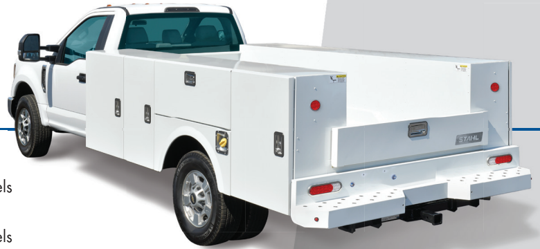
Body pictured with optional Recessed Punched Bumper with surface-mounted LED 3-in-1 Light Kit and Aluminum Fuel Fill
